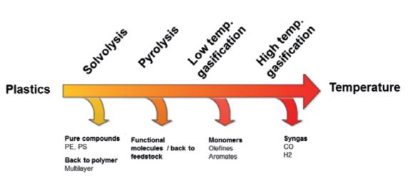
Figure 3-4 Different chemical recycling routes. Based on ECN (2015) [19]
